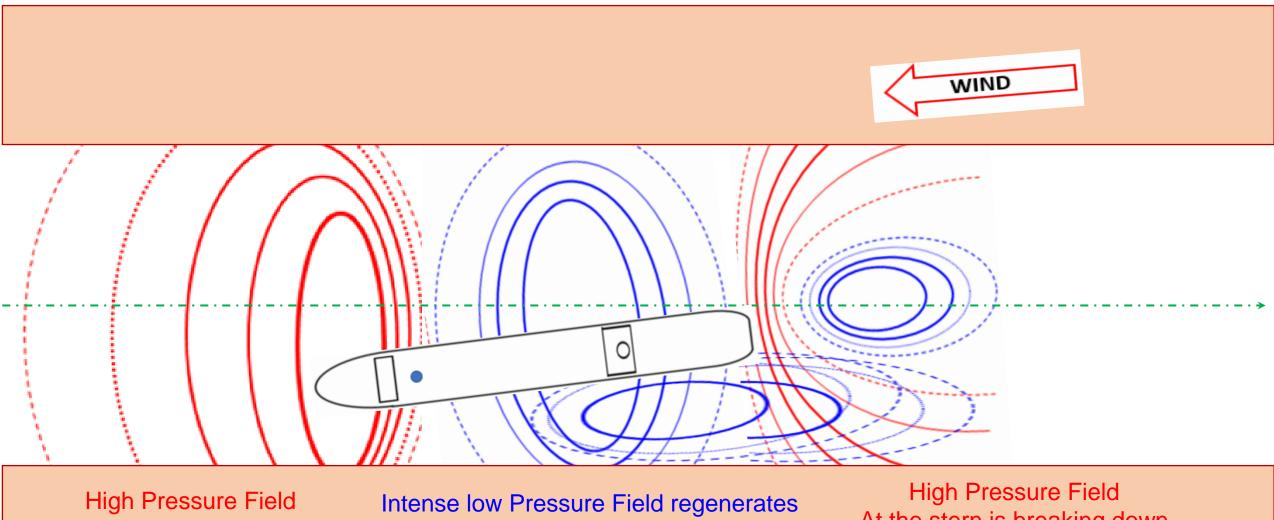
Forcing the bow strongly off the bank ntense low Pressure Field regenerates on the opposite (Port) side and becomes dominant High Pressure Field At the stern is breaking down and no longer helping to keep the stern off the bank
