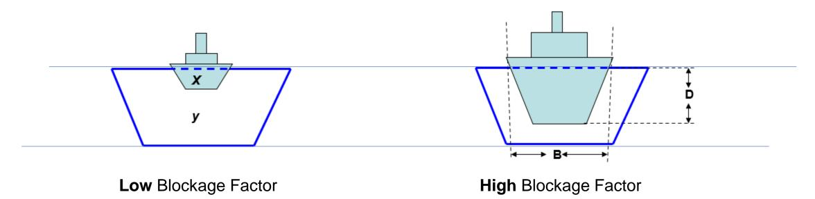
The **BLOCKAGE FACTOR** is the mathematical relationship between and that of the vertical **underwater cross-sectional** of a ship and the vertical **cross-sectional area of the waterway-** usually expressed as a percentage of one against the other.
